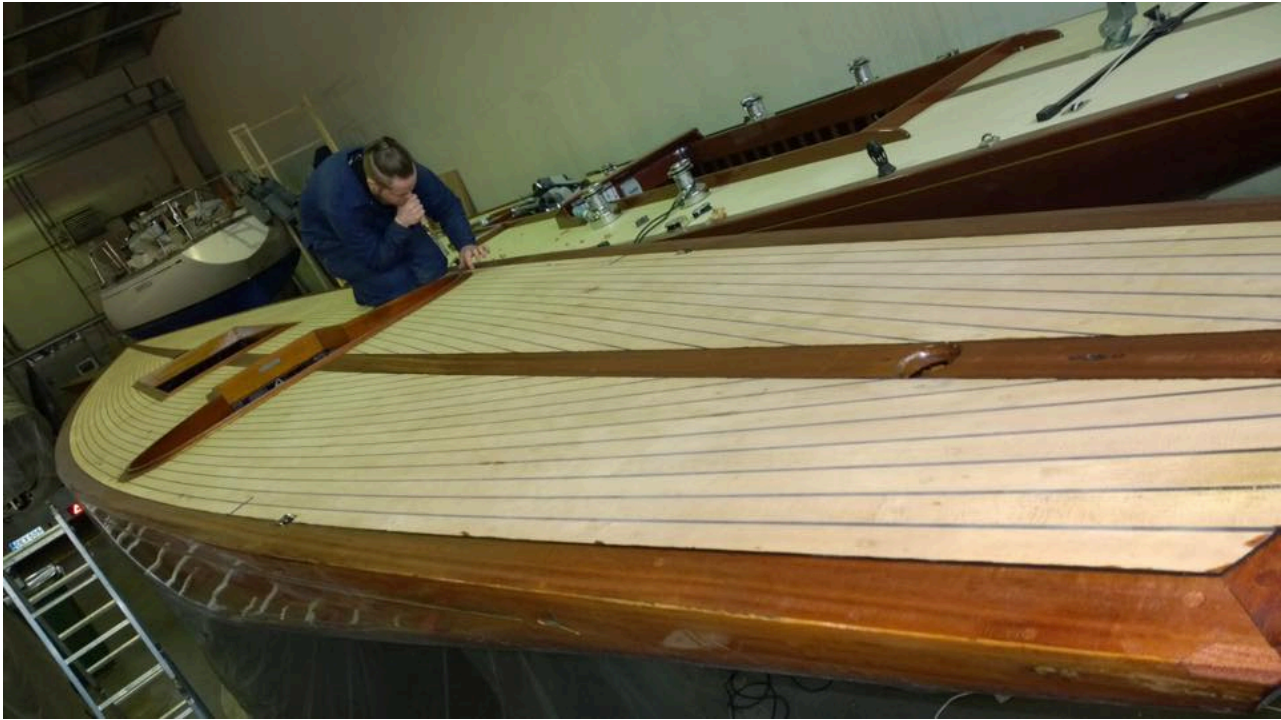
FIN 43 Wire undergoing deck works – FIN 22 Merenneito on the background (Wilenius Båtvarv)
